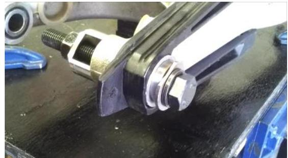
15. Draw in the seal until the large washer stops flush against the outside edge of the bearing housing.
