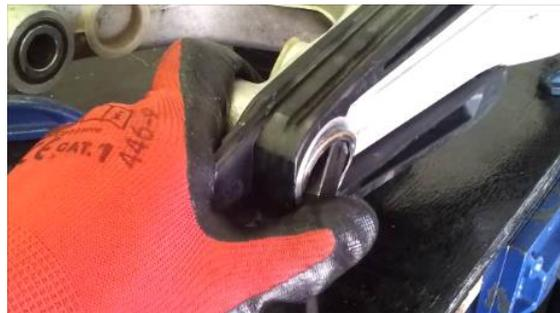
2. Remove the washers. There should be one on each side of the left bearing housing (chain side).
