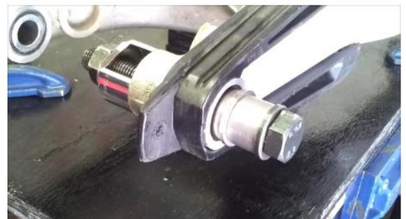
10. Draw in the second bearing until the driver washer stops against the inner lip.
