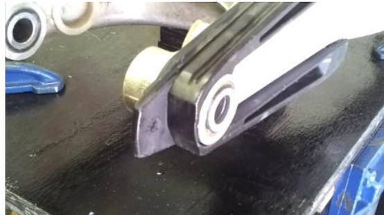
18. One side done. Repeat procedure for the bearings on the other side of the swingarm.
