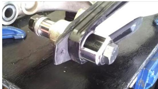
4. **IMPORTANT: Oil the thread and base of bolt head with engine oil.**
